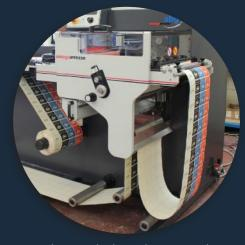
The unwind tension control system combined with the loop control is supported by an ultrasonic sensor to offer smooth operation.
