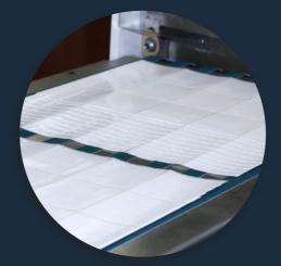
Intersheet double cut allows waste to be removed between sheets.
