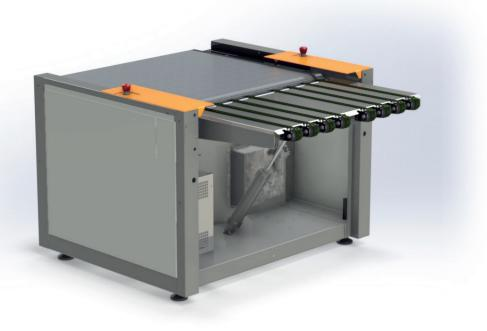
Infeed Module with a pneumatically operated drop-down conveyor fitted with a vacuum hold-down system. The drop-down conveyor allows easy access to the print machine for set-up and cleaning.
