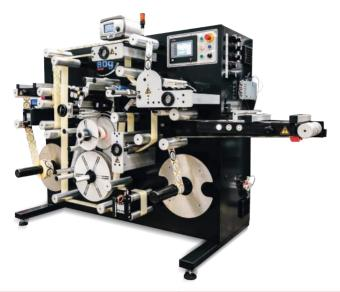
The Ti200 is an entry level machine which takes rolls of finished, printed, die-cut labels and inserts security technology in a single pass. Its ease of use and low investment gives easy access to this exciting and rapidly expanding market.
