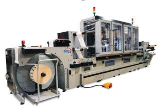
Converting systems for RFID production vary considerably from client to client. The Omega converting line gives customers a wide variety of functions and features to choose from in order to build a converting system that meets with their individual requirements. Converting modules are available in 330mm (13"), 430mm (17") and 530mm (21") web widths and can produce self-adhesive label solutions as well as tag and ticket products.
