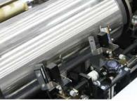
CCD Camera for sheet alignment system
