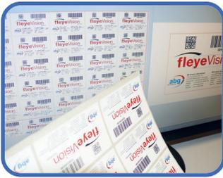
fleyeVision Proof offers a simple possibility to inspect the printing results offline. The digital template will be compared with a sample print from your printing machine or a sample of your received material.
