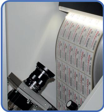
This is usable either as an additional option for the »Standard-print inspection« or without another inspection. In both cases a special line scan camera will be used only for the Braille inspection along with a special illumination and a special new designed software. If braille and »normal« print defects will be inspected, two cameras are necessary.
