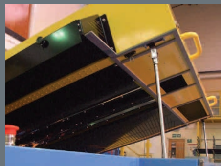
Gas filled lifting arms on the hood
