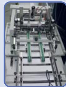
The servo controlled registration system guarantees a high productivity up to 36.000 booklets per hour and a positioning accuracy of +/- 0.5 mm.
